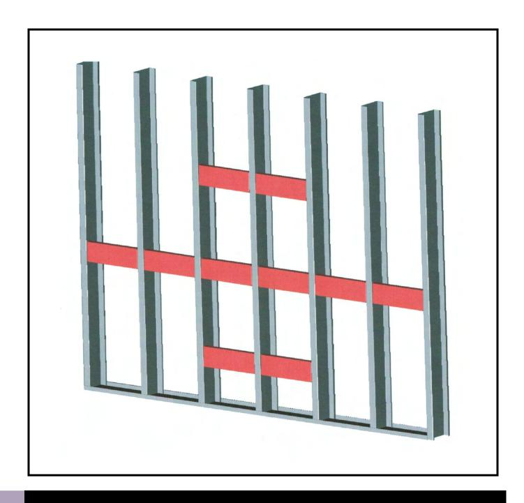
Metal-Lite's patented 3-in-1 backing is the only installation solution for continuous handrails that meet ADA and all nationwide code requirements. This backing system can also be used for the installation of individual applications.
