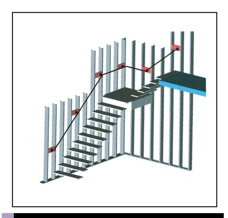
The example above represents the adaptability of Metal-Lites 3-in-1 system. The 3-in-1 can be mounted along both internal and external walls. It can be used in new construction and can also be retro-fitted inside existing walls.
